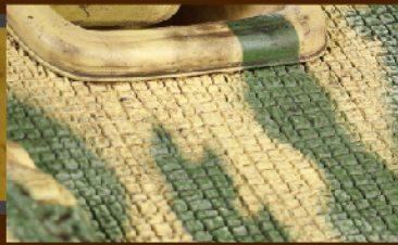
• Realistic square-pattern Zimmerit anti-magnetic mine coating used on early model Jagdpanthers
